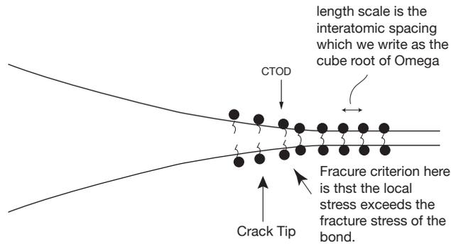
(ii) The crack tip opening displacement (CTOD)
